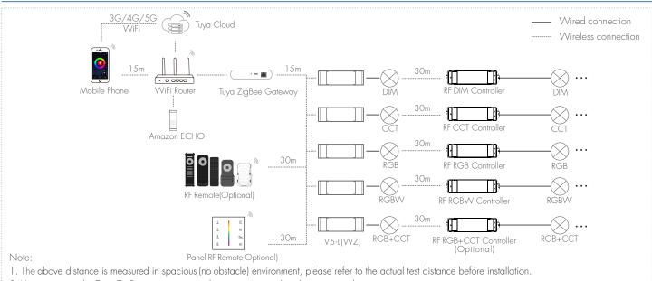
2. Users must use the Tuya ZigBee gateway to realize remote control and voice control
